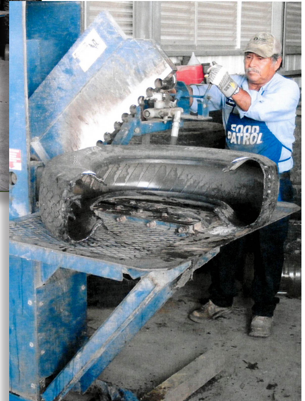
The Starr County Transfer Station purchased tire cutters to provide a smooth method in processing the recycled material.
