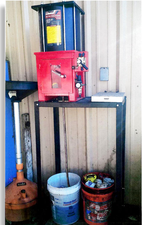
An oil filter crushing apparatus drains any remnant liquid from filters before crushing them.
