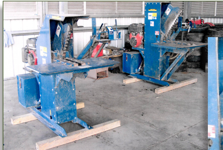
The Starr County Transfer Station purchased tire cutters to provide a smooth method in processing the recycled material.
