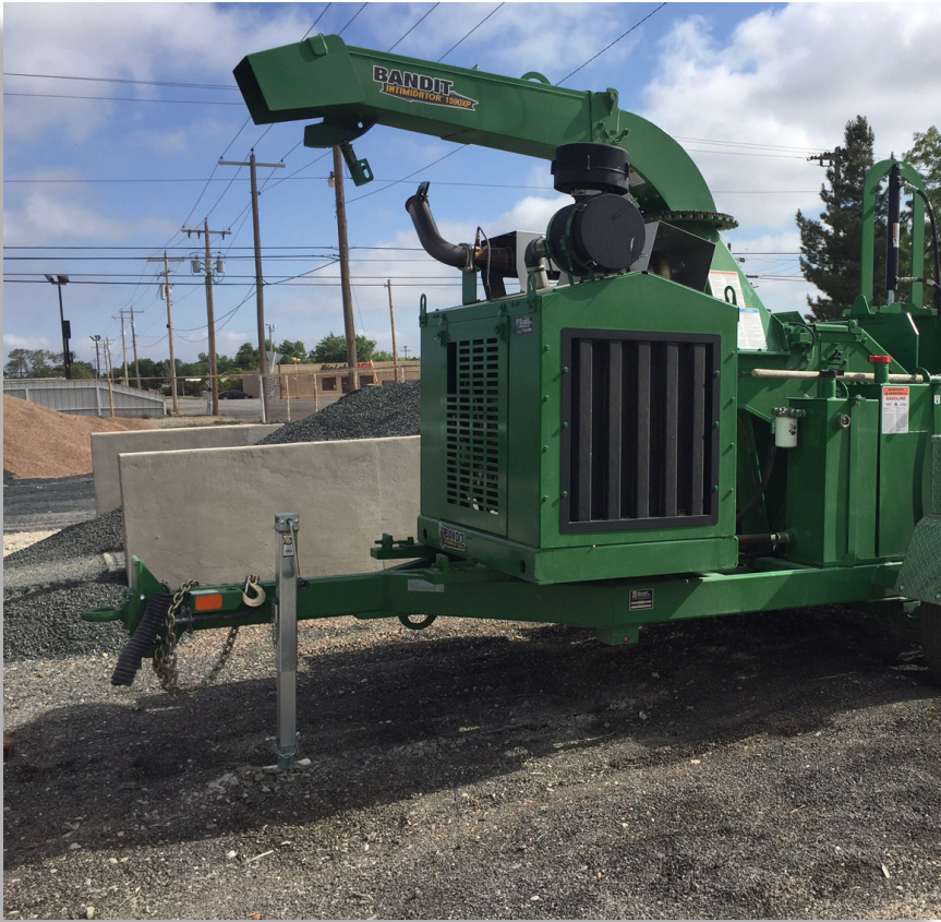
Using a 15-inch Drum Style Brush Bandit (Model 1390XP), the City of Big Lake chips tree limbs, stumps, and vegetation weekly. As a result, a yearly reduction of approximately 53 tons of space has been seen in the city landfill.
